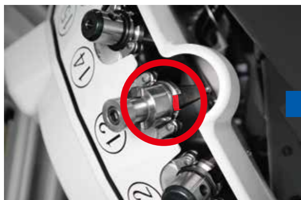
Due to the incorrect tool placement, the drive block doesn't into the drive slot of the holder.
