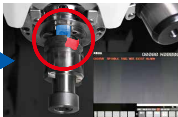
Controller displays alarming messages when the tool doesn't clamp completely.
